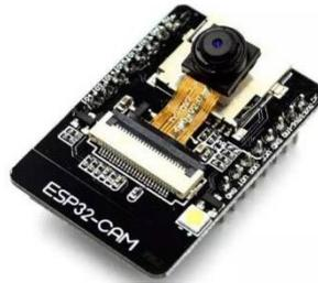
**Gambar 2. Esp32 Cam**
