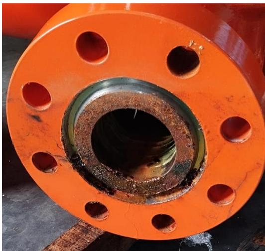
Gambar 1 *Rust damage*
