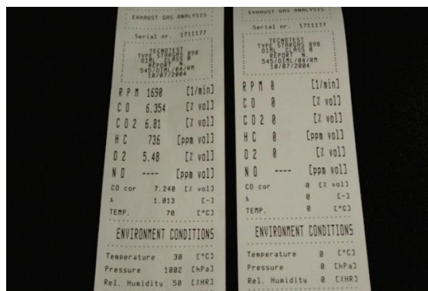
Figure 9. Paper of Emission Test Result from Diesel Aerator and Hybrid Aerator
