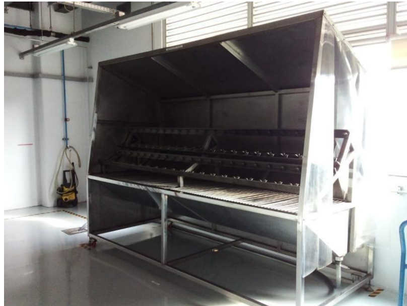
Gambar 2 Filter Cleaning Booth ac
